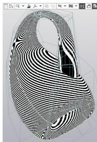
Fig. 28. Testing surface quality using the "Zebra" option.
