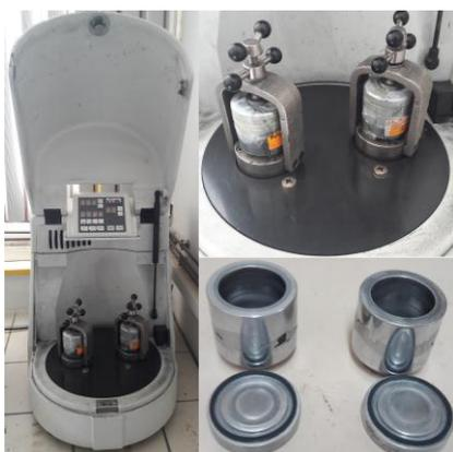
Fig.1. Pulverisette 7 planetary ball mill and vials used in experiment.
