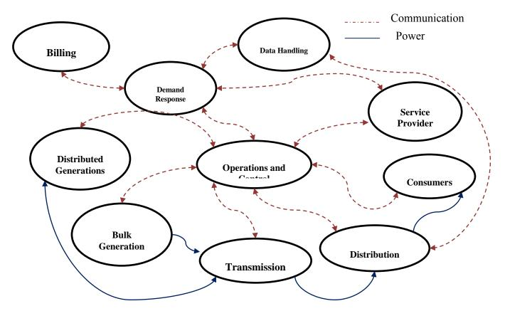
Fig. 2 Typical Layout of Smart Grid
