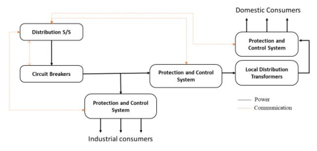
Fig. 3 Layout of Smart Meters
