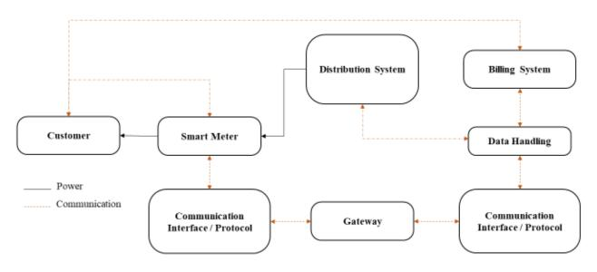
Fig. 3 Layout of Smart Meters
