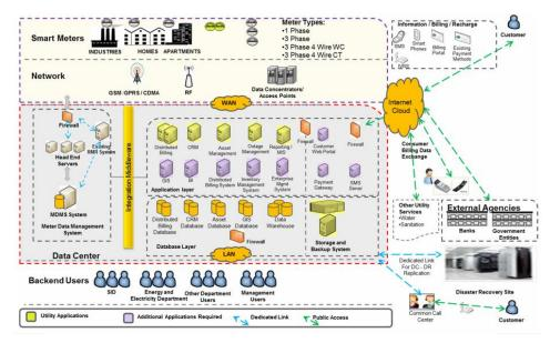
Figure 5. Smart Utility Meter Architecture with IoT [21]
