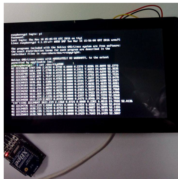
Figure 5: Sample sensor data during monitoring Smart mode sent over Zigbee.
