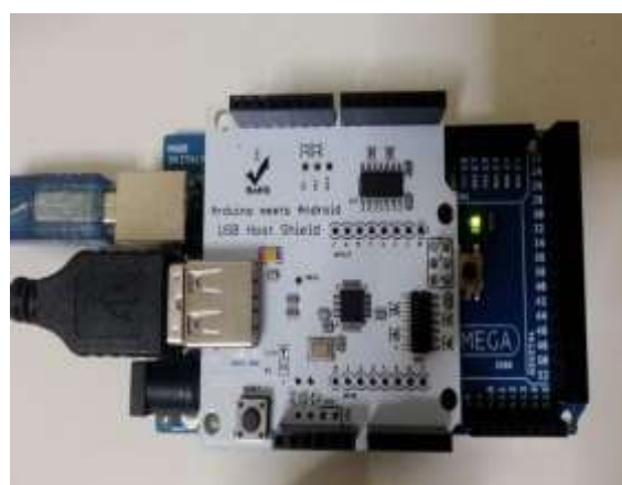
Fig. 6. Arduino mega and usb host shield system architecture
