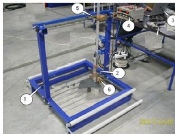
Fig.7 Test bench for testing sheet composite material. 1 - frame, 2 - detector, 3 - spectrometer processor, 4 - power supply, 5 - detector movement carriage, 6 - gamma source movement carriage.
