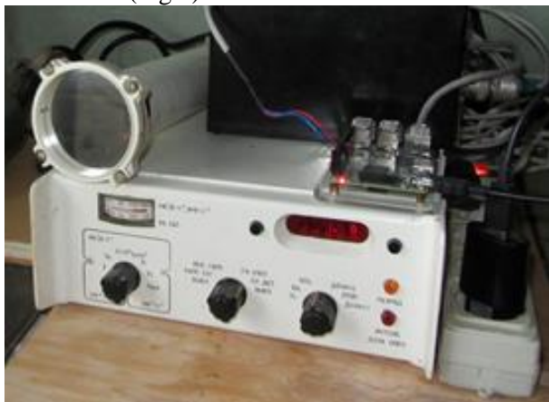
Fig.5 Radiometric system for measuring attenuation of ^{90}\text{Sr}^{(90)\text{Y}} beta source material.
