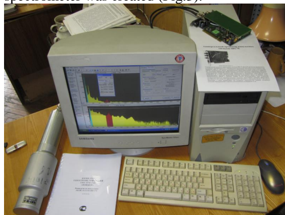
Fig.3 Gamma spectrometer SKS-07P-G41 based on a NaI (Tl) scintillation detector and an SBS-75 pulse signal processor.
