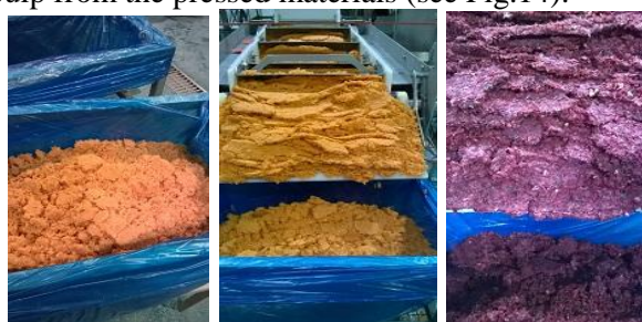
Fig.14 Waste from cold pressing process within the natural juices production
