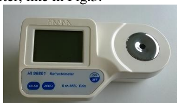
Fig.3. Refractometer for juice sample
