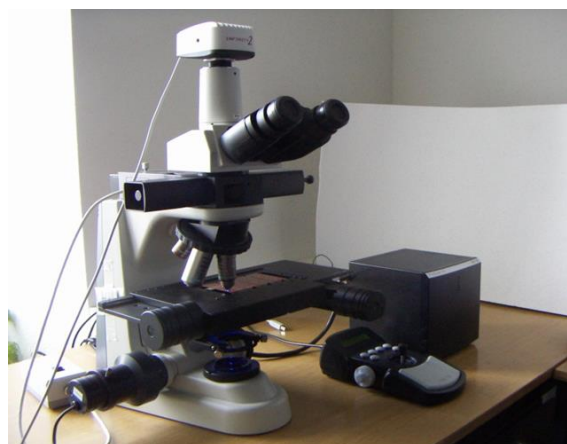
Fig. 5b. Microscope with camera and x-y table
