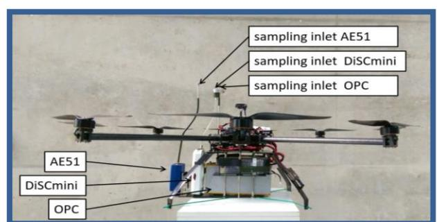
Figure 4: Octocopter with measurement instruments
