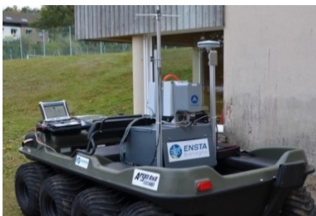
Fig.3. ARGO vehicle with laser scanner (Leica HDS6200), INS (iXSea LandINS) and GNSS receiver (Ashtech Magellan Proflex 500) [6]
