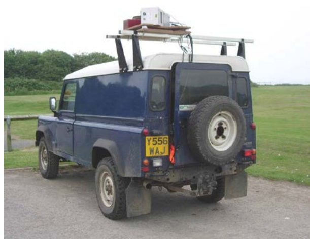
Fig.1. Reigl LMS Q560 airborne lidar system and AEROcontrol GPS/IMU system mounted on the 4x4 vehicle [4]
