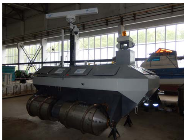
Fig.7. Unmanned ground vehicle for coastal monitoring: setting of the rotary-screw mover
