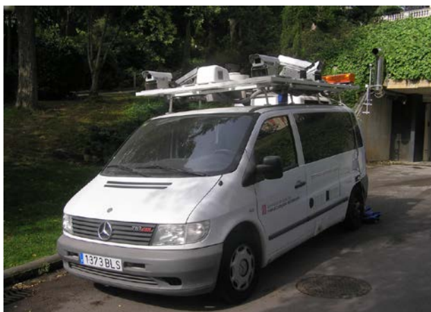
Fig.2. Geomobil (Institut Cartografic de Catalunya) with Riegl LMS Z-210 laser scanner, capable of collecting up to 10000 points/per second, and positioning system belongs to Applanix (POS LV 420) [5]
