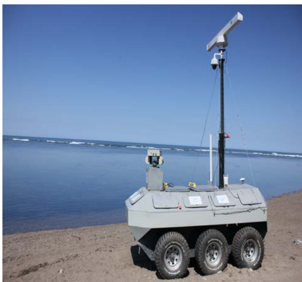
Fig.5. Unmanned ground vehicle for coastal monitoring: wheeled version in the measurement process
