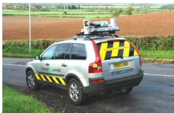
Fig.4. StreetMapper [7]: Inertial system TERRAControl, Up to 4 Riegl LMS – Q120 laser scanners for a 3600 field of scan, Video cameras for a better data interpretation
