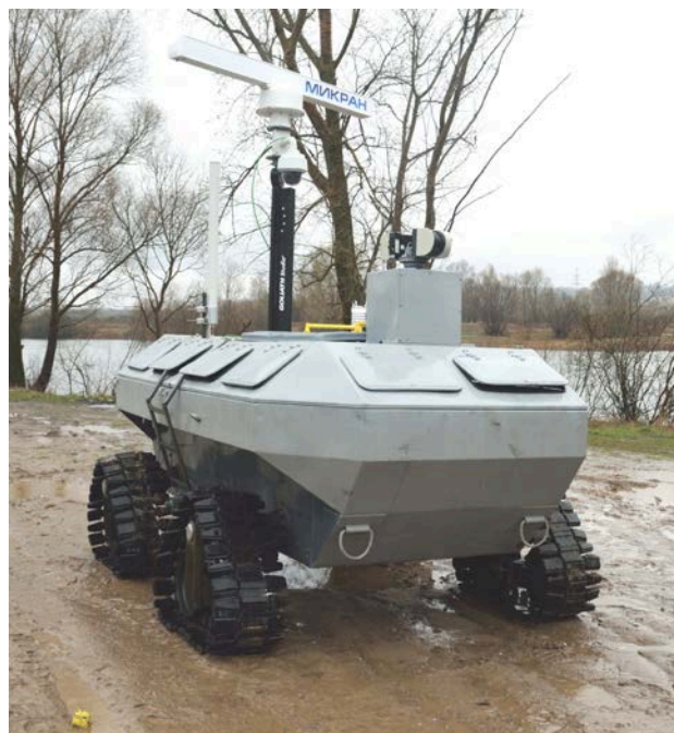
Fig.6. Unmanned ground vehicle for coastal monitoring: tracked version in transportation mode
