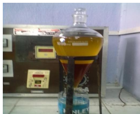
Fig. 3 Settling after base treatment
