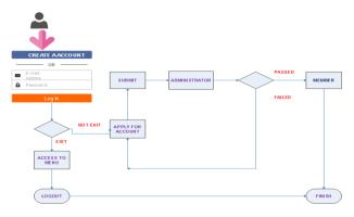
Fig.4 Login diagram for a fresh application.
