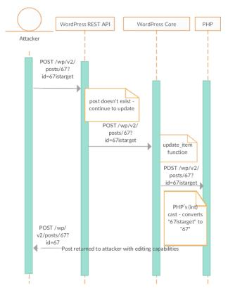
Figure 4. Wordpress REST API attack in 4.7.0 and 4.7.1 versions
