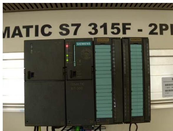
Fig. 2 Diagnostic lights of PLC S7 315F
