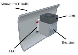
Fig.2 – Thermal module design.
