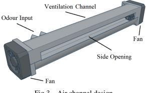
Fig.3 – Air channel design.
