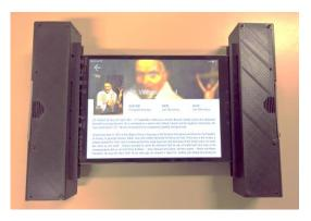
Fig.8 – Portable device assembled with a tablet.
