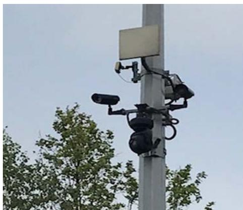
Fig.1 NIR cameras on traffic intersections
