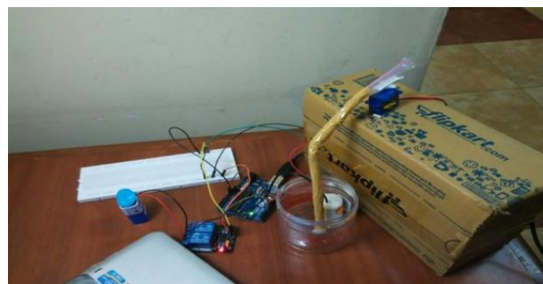
Fig.7. Water spray system setup
