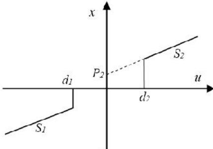
Fig.2b. Hard nonlinearity with preload and dead zone
