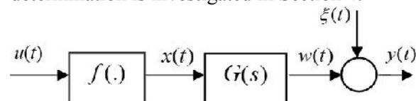
Fig.1. Hammerstein model structure
