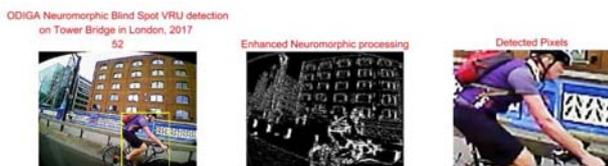
Fig. 10. Neuromorphic CRNN for blind spot cyclist detection, (left) input video frame with yellow box for detected cyclist, (middle) intermediate result of RNN processing, (right) cyclist detection with segmented image
