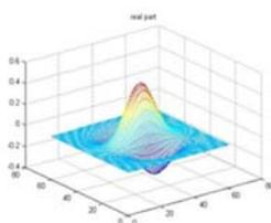
Fig. 6. Gabor complex filter illustrating the orientation feature extraction, in real-part
