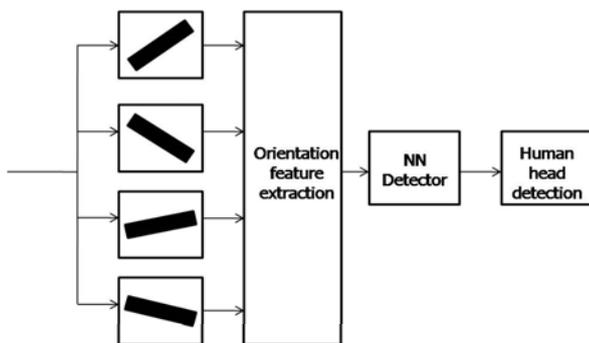
Fig. 2. Neuromorphic visual processing (NVP) for human detection, mimicking the visual cortex neuron
