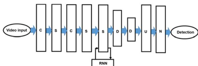
Fig. 5. Neuromorphic convolutional-recurrent neural network (CRNN) for salience-based object detection
