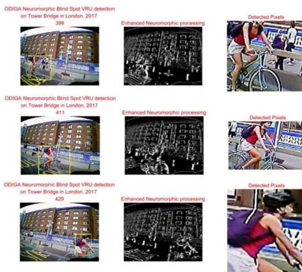
Fig. 12. Neuromorphic CRNN for blind spot cyclist detection for 3 moments over 1 second, (left) input video frames with yellow box for detected cyclist, (middle) intermediate result of RNN processing, (right) cyclist detection with segmented image
