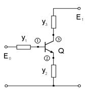
Fig. 6. One-stage transistor amplifier.
