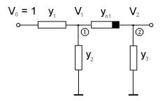
Fig. 1. Two-node nonlinear passive network.
