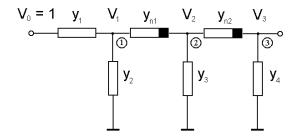
Fig. 4. Three-node nonlinear passive network.
