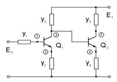
Fig. 8. Two-stage transistor amplifier.
