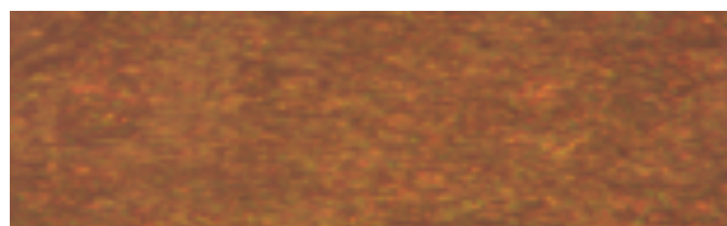
Fig 4 –Structure of copper surface with a porosity of 0.24% after immersion in PGC for 6 hours and kept inside an air sealed box for two days, as viewed under metallurgical microscope in 40 X magnifications. The change in structure and formation of nano porous gold is seen through the microscopic view. Further heating for 2 minutes reduces the resistance to 0.12Ω
