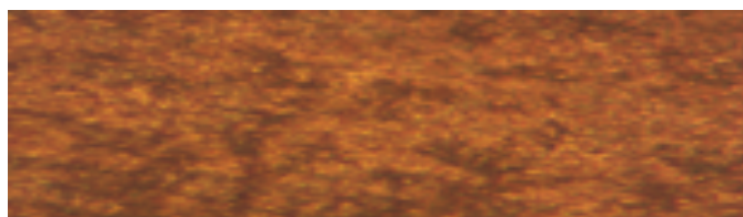
Fig. 3 –Structure of copper surface after immersion in PGC for 2 hours as viewed under metallurgical microscope for 0.24% porosity microscope in 40 X magnifications
