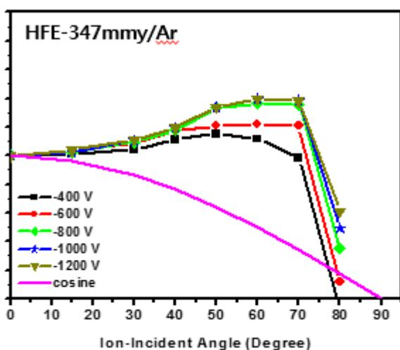
Fig. 5 Angular dependence of normalized etch yields of SiO<sub>2</sub> in HFE-347mmy/Ar plasma at various bias voltages
