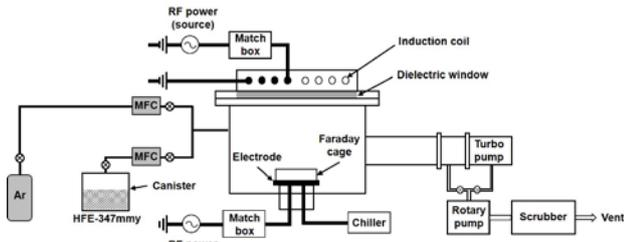
Fig. 1. Schematic diagram of an inductively coupled plasma system.
