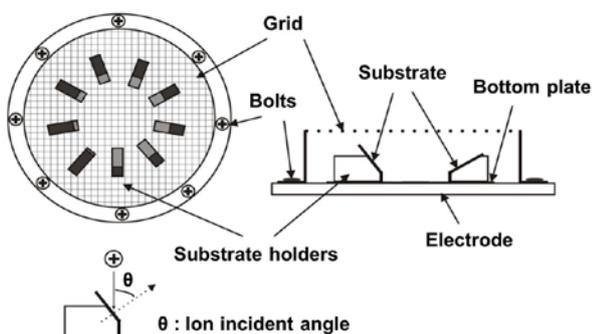
Fig. 2. Schematic diagrams of a Faraday cage and the substrate arrangement in the cage.
