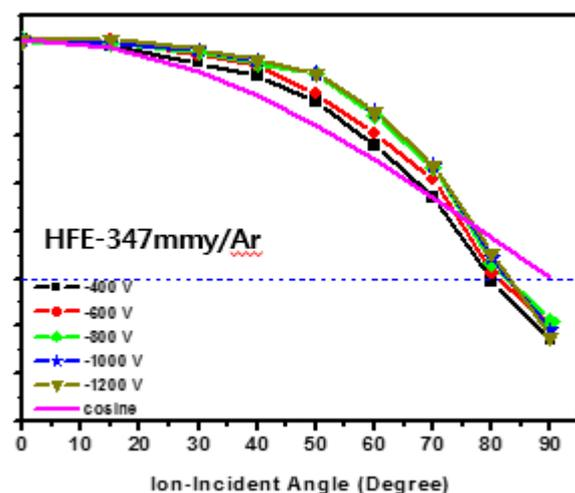
Fig. 4. Angular dependence of normalized etch rates of SiO<sub>2</sub> in HFE-347mmy/Ar plasma at various bias voltages.
