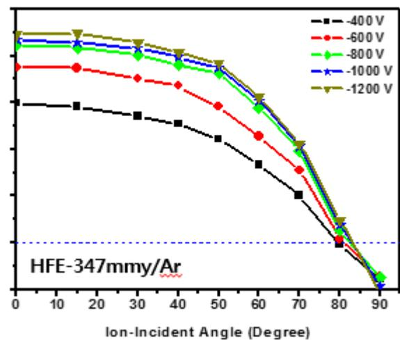
Fig. 3. Angular dependence of etch rates of SiO<sub>2</sub> in HFE-347mmy/Ar plasma at various bias voltages.
