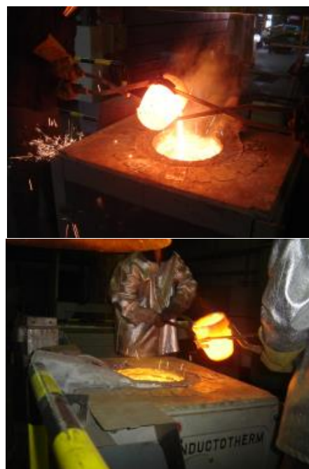
Fig. 2: Images of the process of liquid addition of the alloying elements to the base metal during the tests to evaluate the technical feasibility of the technology.
