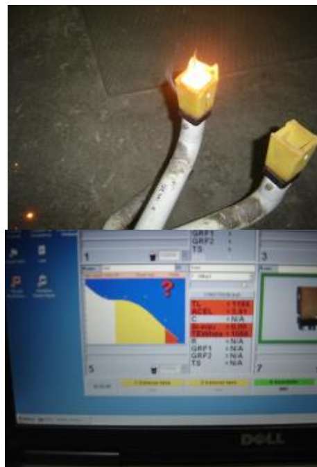
Fig. 1: Images of the liquid temperature determination test using Differential Thermal Analysis techniques.
