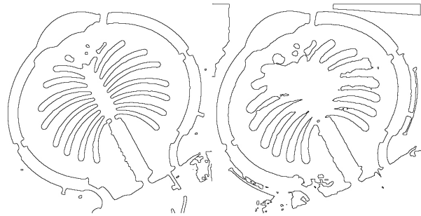
Figure 1: Coastline extraction when histogram matching was turned off (left) and with histogram (right)
