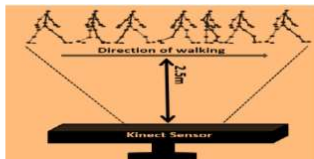
Figure 3: Kinect Sensor Positioning
