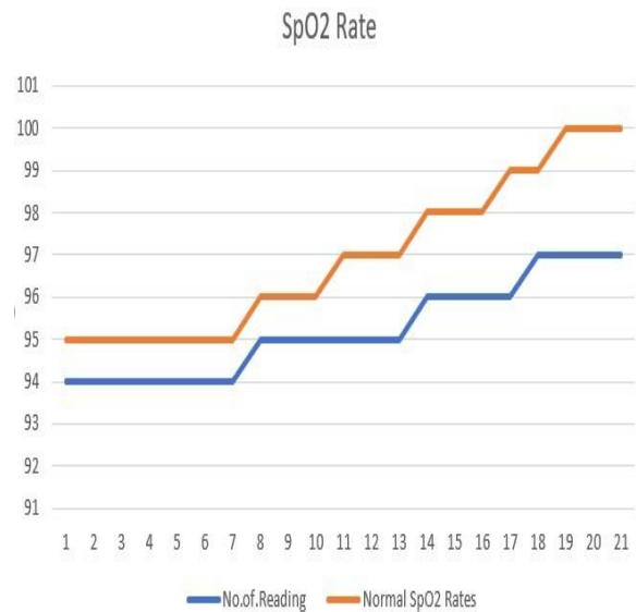
Fig 6 Plots the accuracy of MAX30100(SpO2 level)
