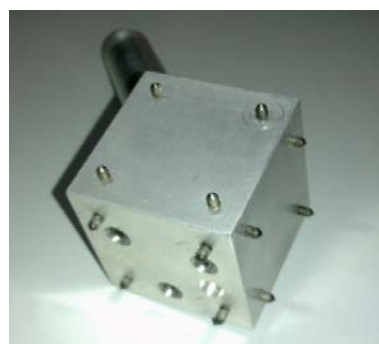
Figure 2: Terminal element of the calibration end-effector
