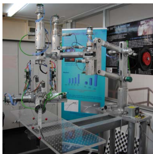
Figure 1: Navi - Robot system: robotic system with 6 DOF
