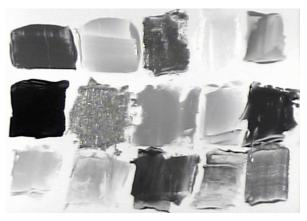
Fig.1b, A photograph of ceramic dyes in NIR (1000 nm) spectrum
