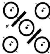
Fig. 2. The thin disks of tetrahedral sites of a Pd lattice where deuterons take place
