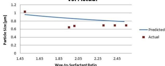
Figure 4 Area Median Particle Size Model compared to Actual Values obtained
