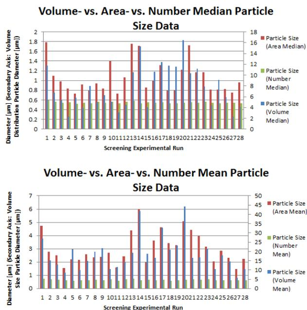
**Figure 2 Particle Size Data (volume-, area- and number particle size data) for all Screening experiments**
