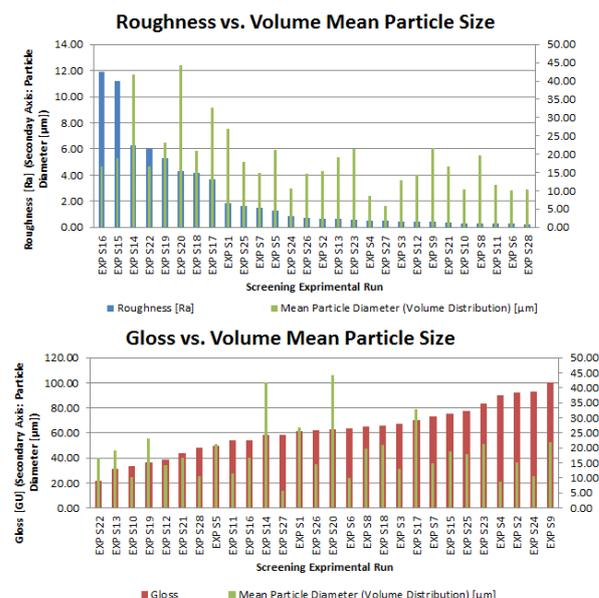
**Figure 3 Roughness- and Gloss Data compared to the Volume Mean Particle Size Data**
