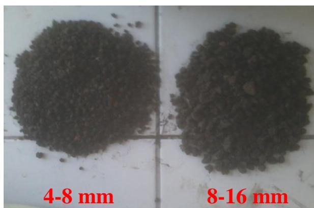
**Fig. 1.** View of basic pumice in 4-8 and 8-16 mm grain size
