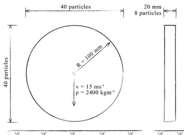
Fig. 2. A diagram of the experiment.
