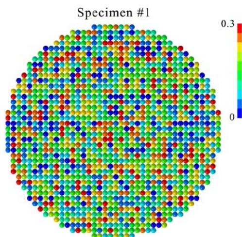
Fig. 5. The mass distribution of specimen #1 (units in g).
