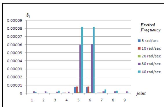
Fig 4. Sensitivity test to excited frequency at 5<sup>th</sup> element of beam (50% reduction of inertia)
