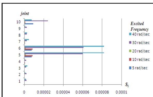
Fig 5. Sensitivity test to excited frequency at 5<sup>th</sup> element of column (50% reduction of inertia)
