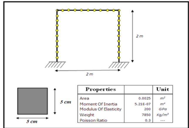
Figure 1. Structural Modelling and Element Properties
