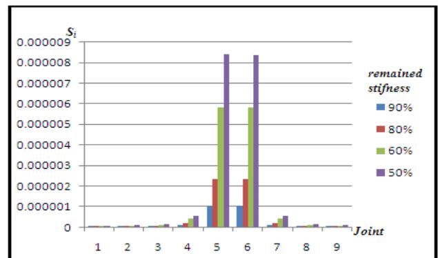
Fig 2. Sensitivity Test: Damage location at 5<sup>th</sup> element of beam (excited frequency 10 radian/sec)
