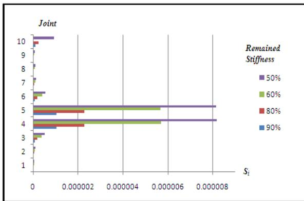
Fig 3. Sensitivity Test: Damage location at 5<sup>th</sup> element of column (excited frequency 10 radian/sec)
