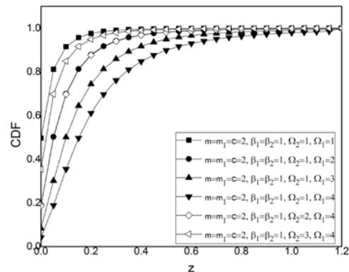
Fig. 1. Outage probability versus output signal to interference ratio  $z$
