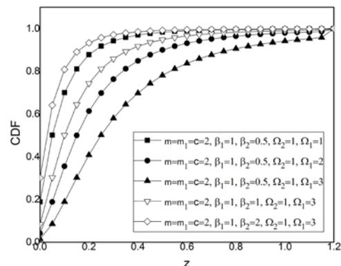
Fig. 2. Outage probability depending on output signal to interference ratio  $z$
