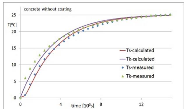
Fig. 3 Measured and calculated temperature evolution in selected points for hardened concrete without coating.
