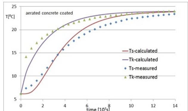
Fig. 2 Measured and calculated temperature evolution in selected points for aerated concrete coated by isolation film.
