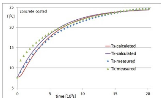
Fig. 4 Measured and calculated temperature evolution in selected points for hardened concrete coated by isolation film.
