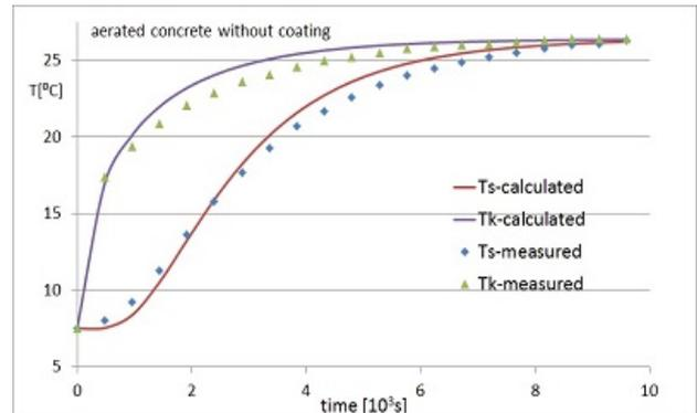
Fig. 1 Measured and calculated temperature evolution in selected points for aerated concrete without coating.
