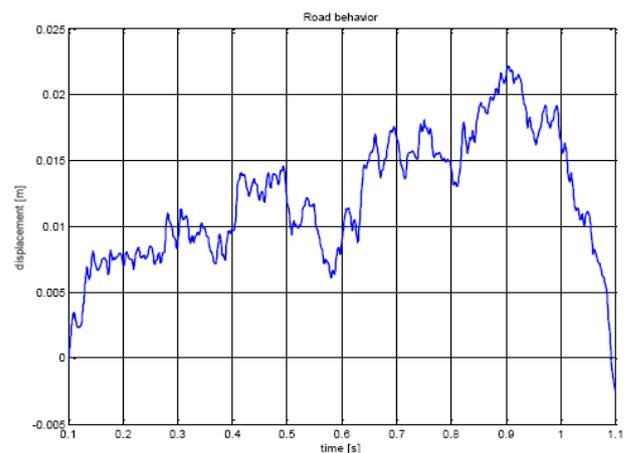
Fig. 7: Random signal approximation used to simulate road displacement
