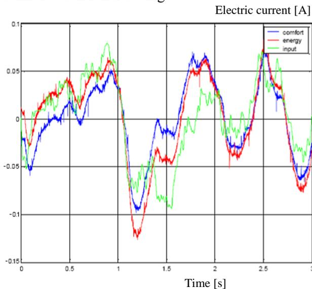
Fig. 10: Demands on electric current as an indicator of energy demands for “energy” and “comfort” controller settings
