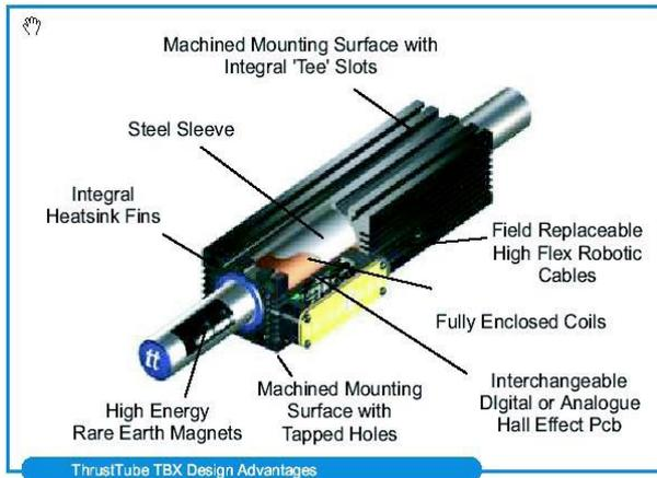
Fig. 3: Linear electric motor - basic structure
