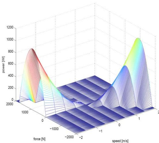
Fig. 6: Force-velocity profile of the recuperated energy of the used linear motor
