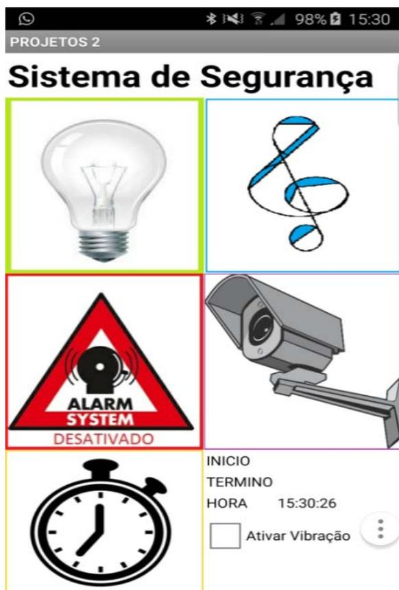
**Fig. 2.** Capture of the app’s initial screen. From top to bottom, left to right: the title: “Security System”, the light bulb activation button, the music player icon, the alarm activation button, which reads: “Alarm System Deactivated”, an IP camera button for future system expansions, the icon for programming the initial and final moments of the simulation of presence and a last tile with information that reads: “Beginning”, “End”, “Time”, “Activate Vibration”.
