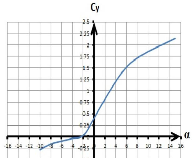
Fig. 4 Graphic of  $C_y$  obtained using CFD
