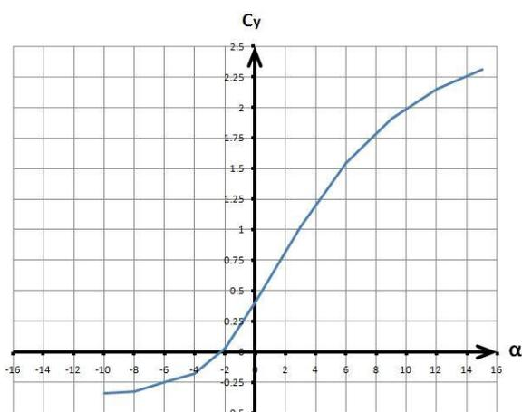
Fig. 3 Graphic of  $C_y$  experimentally obtained
