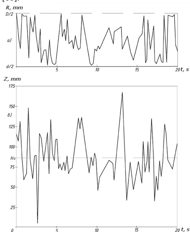
Figure 2. Projections of the particle trajectories in: a) horizontal, and b) a vertical planes at a velocity  $W = 1.5W_{cr}$  and the initial bed height  $H_0 = 0.5D$ .
