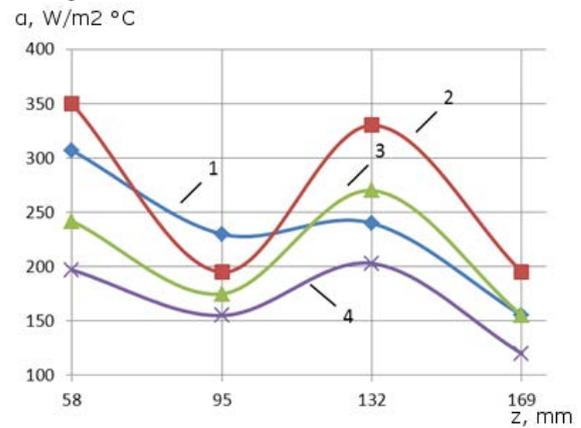
Figure 5. Variation of a coefficient of heat transfer from the bed of silica-alumina catalyst particles (average diameter 2.5 mm) to the vertical cylindrical heater 42 mm in diameter versus the fluidization number  $N$ : 1 –  $N = 1.5$ , 2 –  $N = 2.5$ , 3 –  $N = 3.5$ , 4 –  $N = 4.5$ . Reproduced from data of the work [8].
