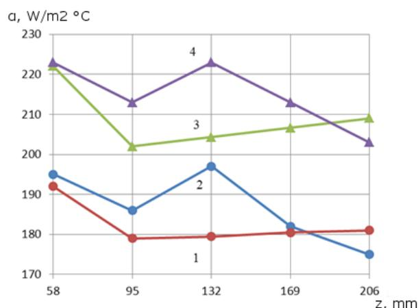
Figure 1.  $\alpha_r$  versus the height of the body in the presence (curves 1 and 2) and in the absence (curves 3 and 4) of the screen tube.
