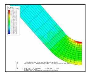
**Fig.4** Von-Mises stresses of [90<sub>8</sub>], geometry of half a section of a U-shaped laminate after demoulding
