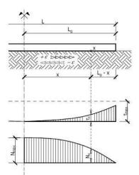
Fig. 10: Shear stress and normal force caused by friction in footing bottom
