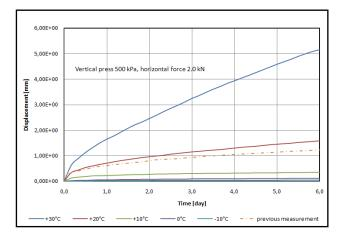
Fig. 7: Measured displacement, influence of temperature
