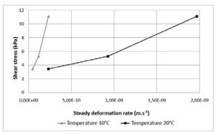
Fig.11: Shear stress as a function of deformation rate
