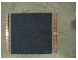
Fig. 5: Electric resistance wire between two layers of asphalt belt
