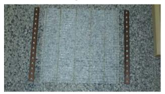
Fig. 6: Electric resistance wire prepared on plastic netting
