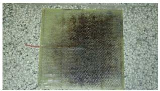
Fig. 4: Electric resistance wire between plastic layers
