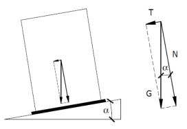
Fig. 1: Primary testing of sliding joint
