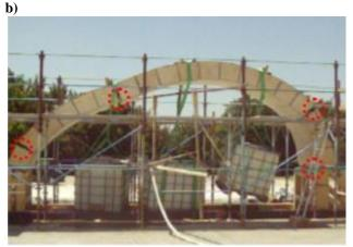
Fig. 2 Tested arch. a) details with the low tanks of the positioning of the displacement transducers; b) collapse mechanism and achievement of the hinges in the arch with an asymmetric load condition.
