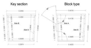
Fig. 1 Executive drawings of the blocks with the connecting system by mean of male-female joints.
