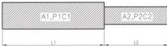
Fig.7: The general case of a plane of stress discontinuity
