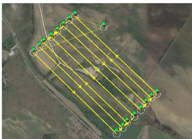
Fig. 1. The flight plan of the area, where recording is intended to take place (Mission Planner)
