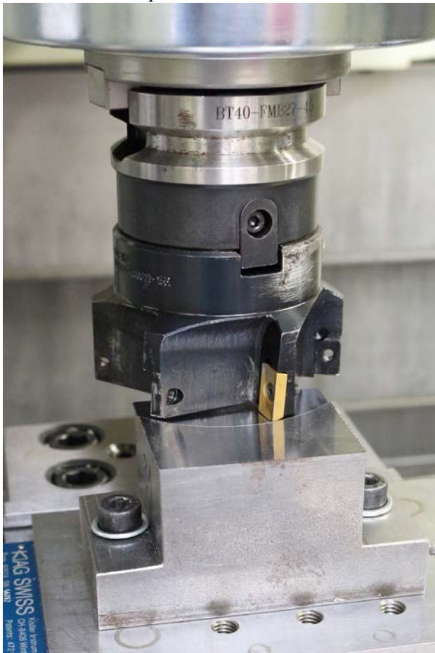
Fig. 1 Milling head with one insert and the workpiece, which is mounted on the dynamometer
