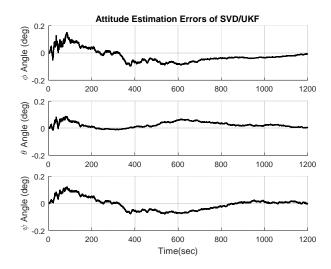
Fig. 4. Attitude estimation errors of SVD/UKF method.
