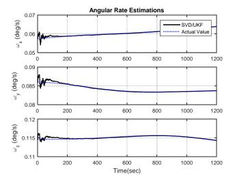
Fig. 5. Attitude rate estimation of the SVD/UKF algorithm with respect to actual simulation values.
