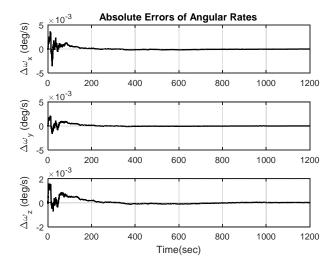
Fig. 6. Angular rate estimation errors of SVD/UKF method.
