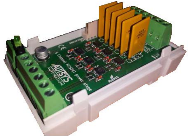
Fig.9 MOSFET power stage
