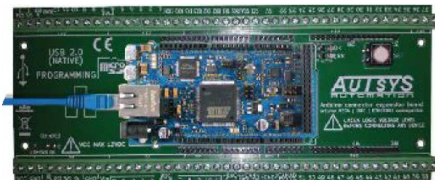
Fig.7 PCB with socket for EtherDue
