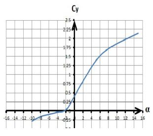
Fig. 4 Graphic of C<sub>y</sub> obtained using CFD
