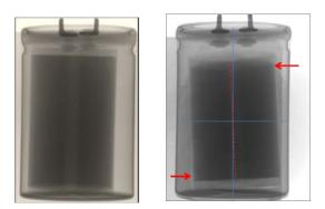
*Fig. 3 X-RAY – of investigated electrolytic capacitors* (*left – original part, right – suspicious sample*
