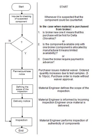
Fig. 1 Flow chart for counterfeit component detection
