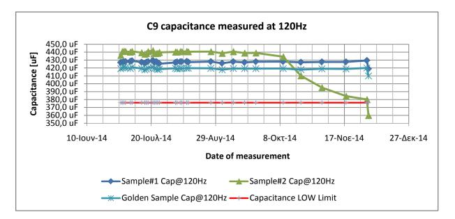
Fig. 11 Dependency of capacitance value on the date of the measurement during dynamic behavior test (120 Hz)
