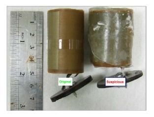
Fig. 6 Encapsulated capacitors for foil reel measurement
