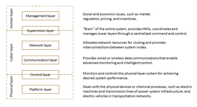
Fig. 5 Hierarchical structure of cyber-physical control systems [19]
